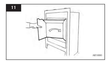
7.2 Check that the panel is sitting behind the rear ledge, but in front of the spacer bracket so that it locates in the slot, Diagram 12.
